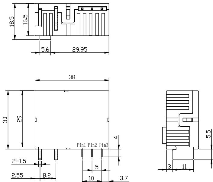
Note: Some product dimensional tolerance is not specified. When <1mm, the tolerance is ±0.2mm; when between 1~5mm, the tolerance is ±0.3mm; when >5mm, the tolerance is ±0.4mm.
