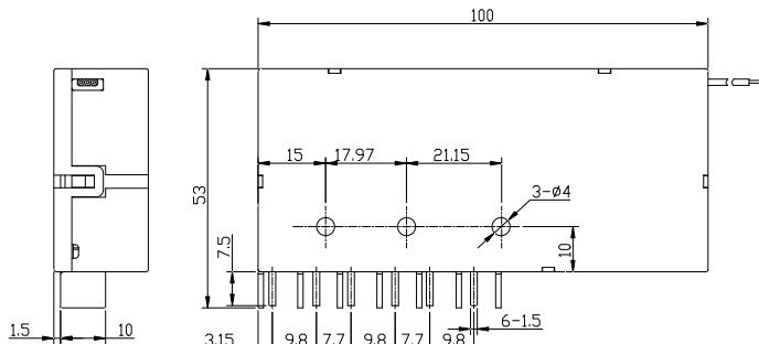
Note: Some product dimensional tolerance is not specified. When < 1mm, the tolerance is ±0.2mm; when between 1~5mm, the tolerance is ±0.3mm;
