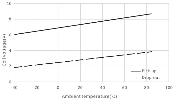
(1)Coil supplied voltage 12VDC;
