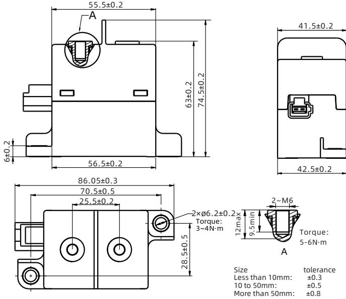
1) Maximum torque is allowed to be installed as shown, only one-time installation is allowed, and repeated tightening of screws is not allowed.
