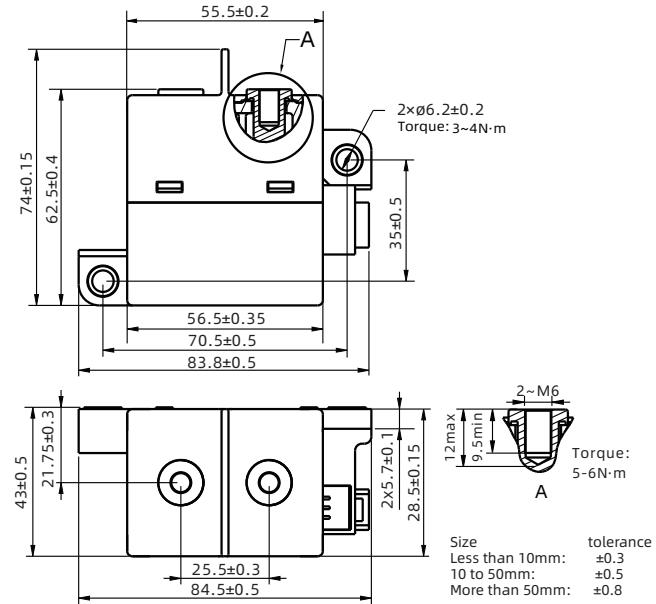
1) Maximum torque is allowed to be installed as shown, only one-time installation is allowed, and repeated tightening of screws is not allowed.
