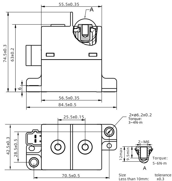
1) Permitted torque 6Nm max. One-time mounting only, no recurring screw fastening permitted.
