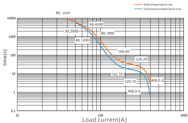
1) The upper limit of safety temperature is 180°C, and the upper limit of functional temperature is 150°C.
