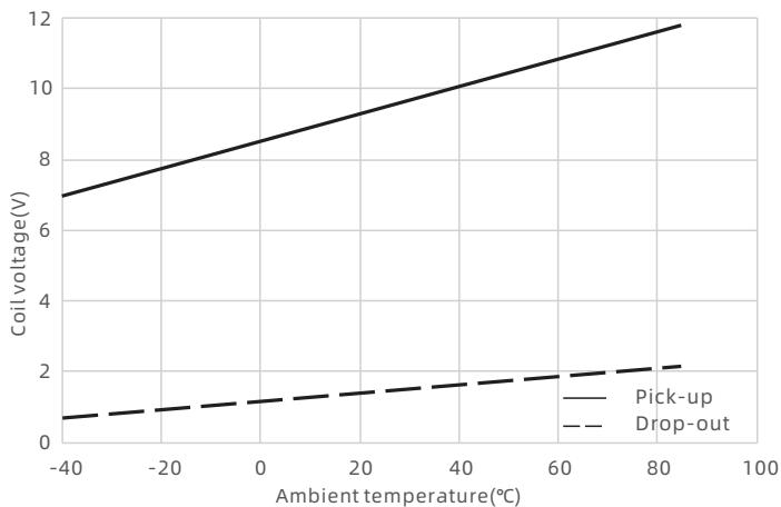
1) Coil supplied voltage 12VDC.
