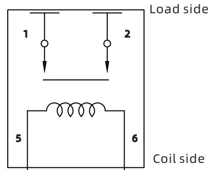
Note: No polarity on load side
