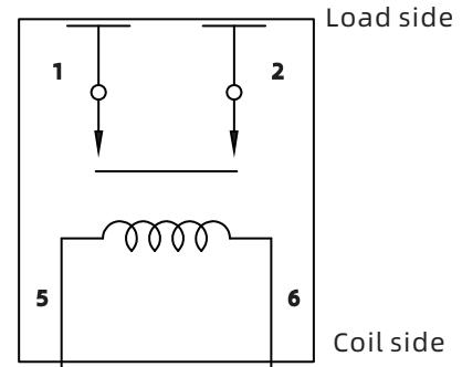
Note: No polarity on load side
