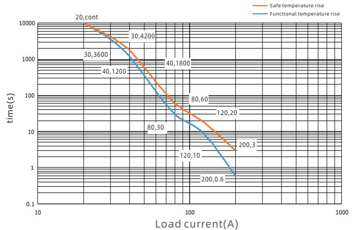
1) The upper limit of safety temperature is 180°C, and the upper limit of functional temperature is 150°C.
