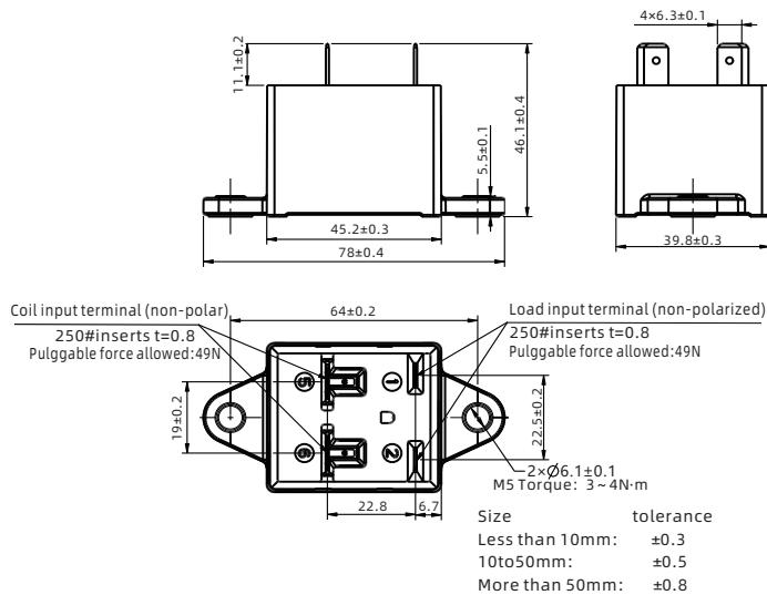
1) Maximum allowable torque as shown in the figure. One-time mounting only, no recurring screw fastening permitted.
