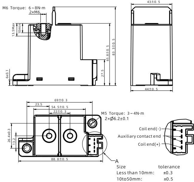
1) Maximum allowable torque as shown in the figure. One-time mounting only, no recurring screw fastening permitted.
