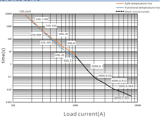
1) The upper limit of safety temperature is 180°C, and the upper limit of functional temperature is 150°C.
