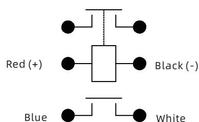
Note: The load end is not polar, and the coil terminal is polar
