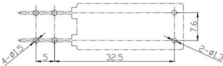
P.C.B. Layout (bottom view)
