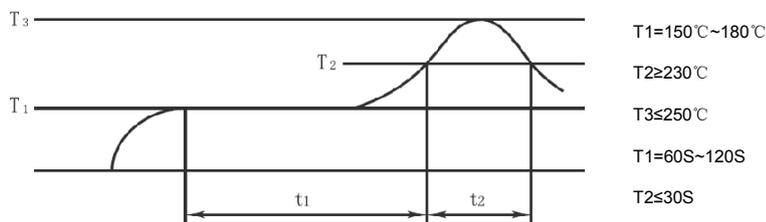
Rise in relay temperature depends greatly on the component mix on a given PC board and the heating method of the reflow equipment. Therefore, please test beforehand using actual equipment to ensure that the temperature where the relay terminals are soldered and the temperature at the top of the relay case are within the conditions given above.
