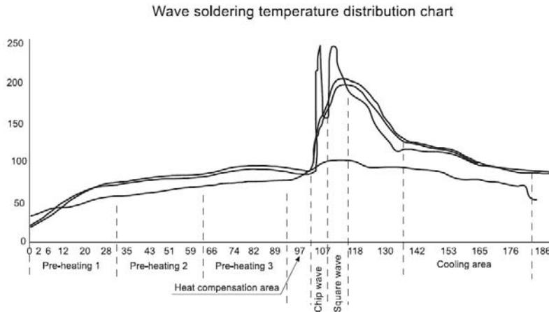
Pre-heating: within 150 °C(solder surface terminal portion)and within 150 seconds.
